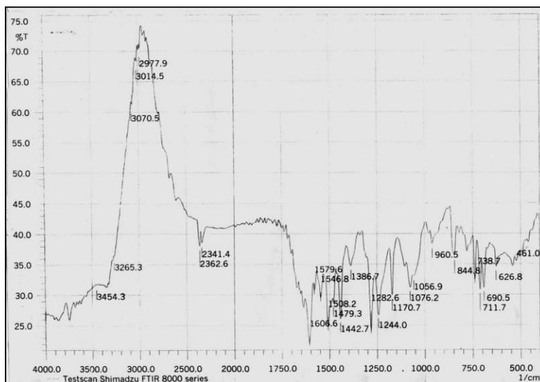
Figure (15): FT-IR spectrum of tri-[4-(5-phenyl-1,3,4-oxadiazol-2-yl)phenyl]phosphate [14].
