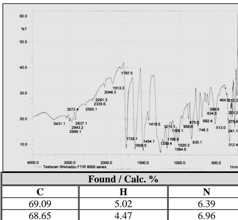
Figure (3): FT-IR spectrum of 2-(4-methoxyphenyl)-5-[4-(*p*-methoxybenzoyloxy)phenyl]-1,3,4-oxadiazole [3].
