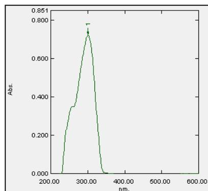
Figure (7): The ultraviolet visible spectrum for 2-(4-methoxy phenyl)-5-[4-(4-methoxy benzoyloxy)phenyl]-1,3,4-oxadiazole [3].
