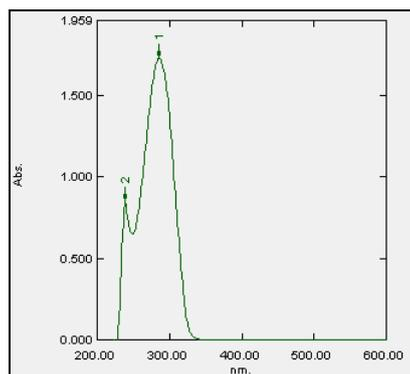
Figure (6): The ultraviolet visible spectrum for 2-(phenyl)-5-[4-(benzoyloxy)phenyl]-1,3,4-oxadiazole [2].
