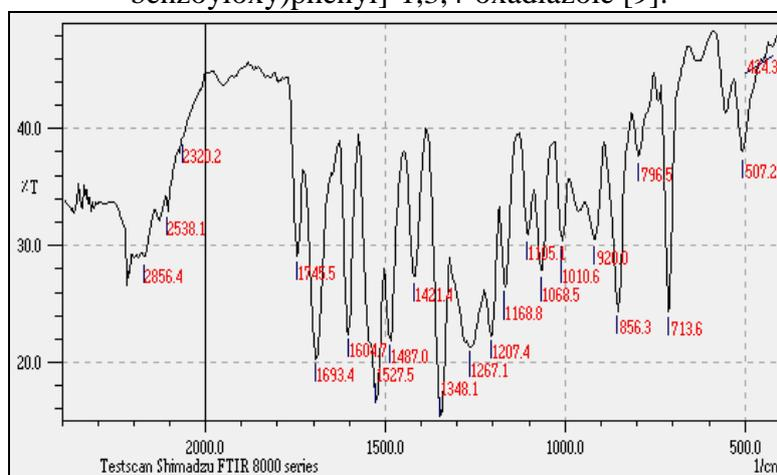
Figure( 5): FT-IR spectrum of 2-(4-nitro phenyl)-5-[4-(4-nitro benzoyloxy)phenyl]-1,3,4-oxadiazole [10].
