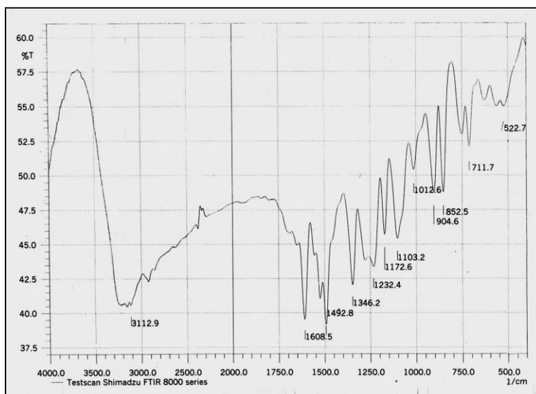
Figure (17): FT-IR spectrum of tri-[4-(5-(*p*-nitro phenyl)-1,3,4-oxadiazol-2-yl) phenyl] phosphate [16].
