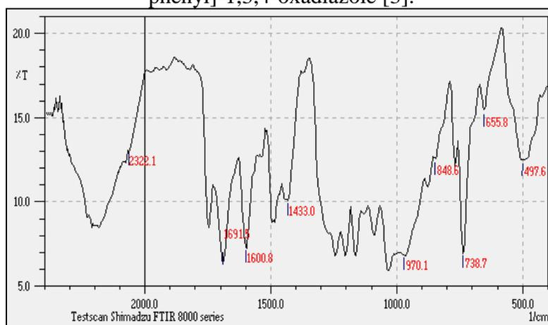
Figure (4): FT-IR spectrum of 2-(2-chloro phenyl)-5-[4-(2-chloro benzoyloxy)phenyl]-1,3,4-oxadiazole [9].
