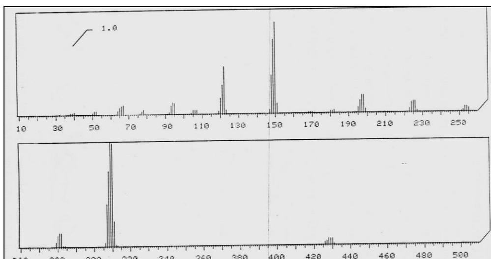
Figure (10): mass spectrum of 2-(*p*-Ethoxyphenyl)-5-[*p*-(4-ethoxybenzoyloxy)phenyl]-1,3,4-oxadiazole [4].
