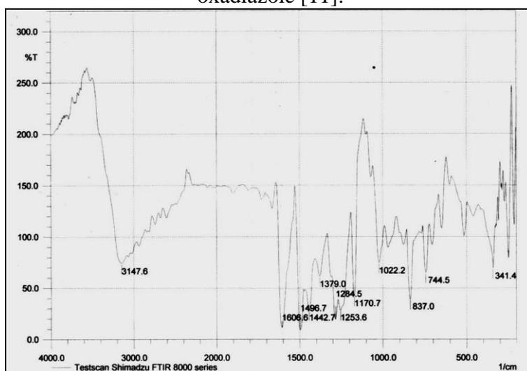
Figure (12): FT-IR spectrum of 2-(4-methoxyphenyl)-5-(4-hydroxyphenyl)-1,3,4-oxadiazole [12].
