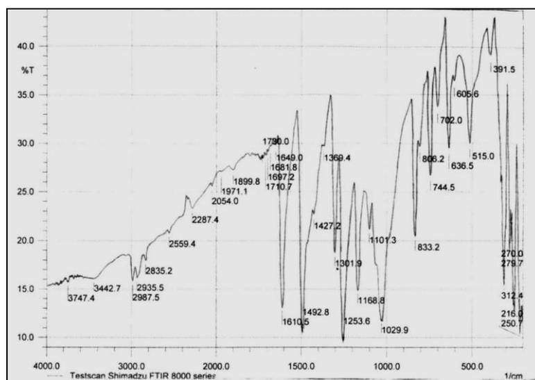
Figure (16): FT-IR spectrum of tri-[4-(5-(*p*-methoxyphenyl)-1,3,4-oxadiazol-2-yl)phenyl] phosphate [15].
