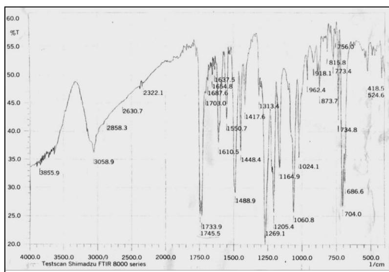
Figure (2): FT-IR spectrum of 2-phenyl-5-[4-(benzoyloxy) phenyl]-1,3,4-oxadiazole [2].
