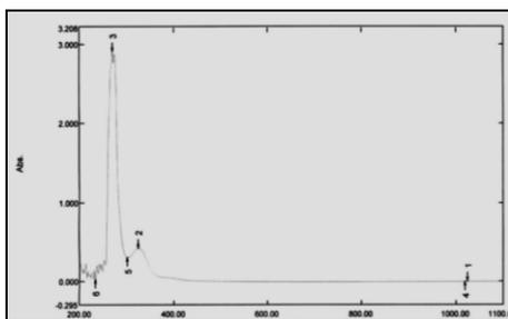
Figure (14): Ultraviolet spectrum of 2-phenyl-5-(4-hydroxyphenyl)-1,3,4-oxadiazole [11].
