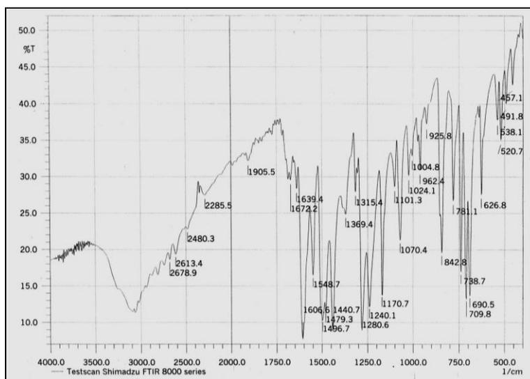
Figure (11): FT-IR spectrum of 2-phenyl-5-(4-hydroxyphenyl)-1,3,4-oxadiazole [11].
