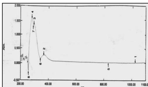
Figure (18): Ultraviolet spectrum of tri-[4-(5-phenyl-1,3,4-oxadiazol-2-yl) phenyl] phosphate [14].
