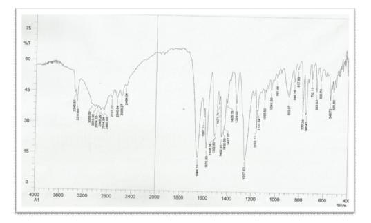
Fig.(2) FT-IR spectrum for prepared imidazole polymer P2
