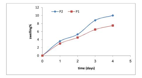
Fig.(4) swelling % of imidazole polymers P1 &P2
