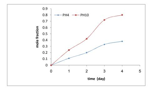
Fig.(3) controlled release of imidazole polymer P1
