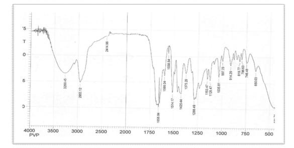
Fig.(1) FT-IR spectrum for prepared imidazole polymer P<sub>1</sub>
