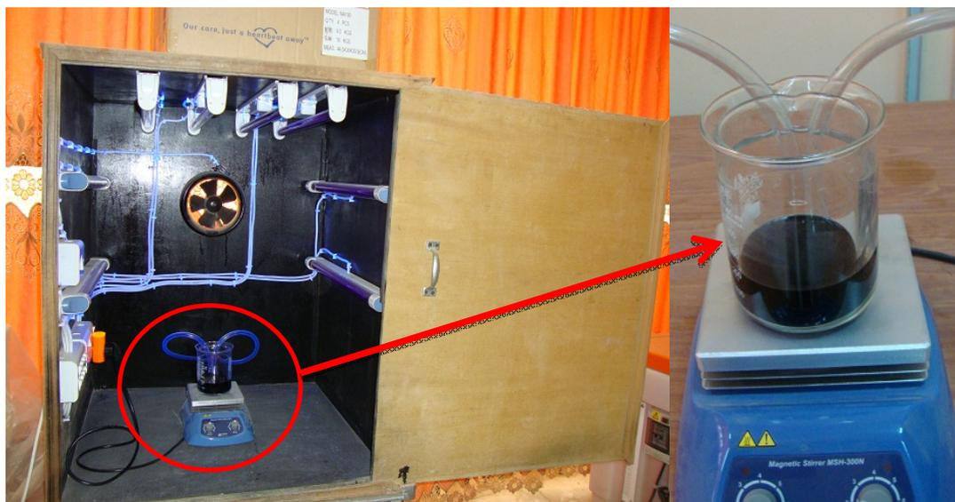
Figure (2): Photocatalytic Chamber and reactor vessel
