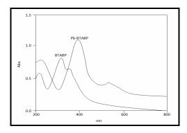
Fig(2): UV-Vis. Spectrum for ligand BTABP & its complex Pb-BTABP as cloud point
