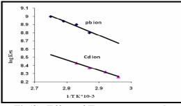
Fig(8): Effect of Temperature on kex
