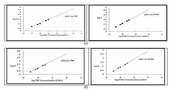
Fig(12): Synergistic effect on D values (a)pb<sup>2+</sup> (b)Cd<sup>2+</sup>ions
