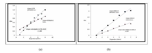
Fig(10): Slope ratio method (a)for pb2+ ion ,(b)for Cd2+ ion
