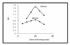
Fig(9): (a) Effect of time of heating on cloud point formation and extraction method
