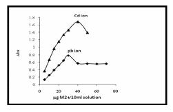
Fig(5): Effect of metal ion Concentration on complex formation by CPE
