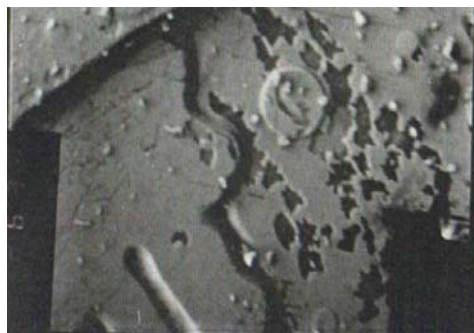
Fig. 4. Single phase alloy made from melting pre-form alloy with CNT
