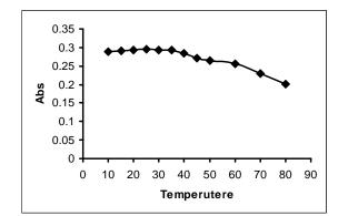
Fig(4) Effect of temperature on stability of complex
