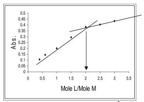
Fig(5); Mole ratio plot [Reag]=[Co<sup>2+</sup>] =3x10<sup>-4</sup>,pH~6.1
