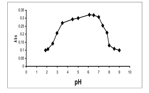
Fig(2);Effect of pH on the absorbance of Co- (6-MeBTACIP) complex
