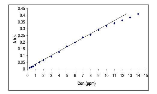
Fig(7); Calibration curve of Co (II) - (6-MeBTACIP) complex
