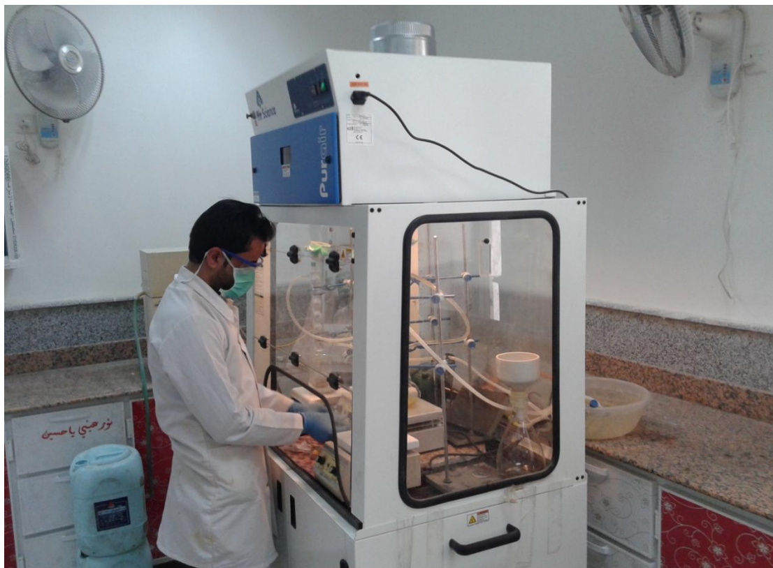
Figure 4: Safed conditions of chemical hood for laboratory user at faculty of science-University of Kufa
